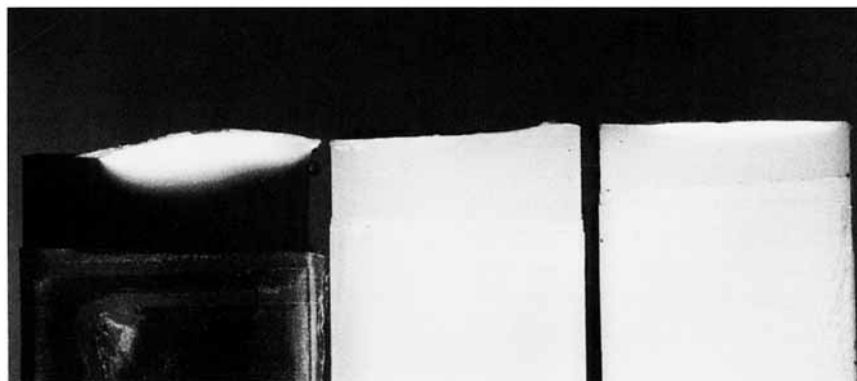
Figure 7 Optical micrograph of stress-whitened zone, from left to right: PA11/NBR(LAN) : 80/20 blend, HIPS, and ABS.
